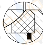
DETAIL - Y FIRE SAFE DESIGN
